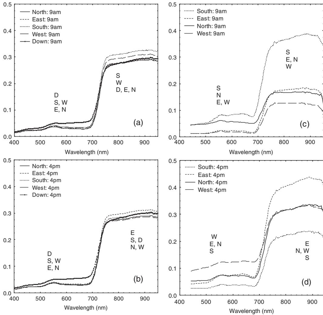
Fig. 5. Comparison of reflectance spectra calculated for four azimuths using the Kuusk (1995) model at (a) 9:00 AM and at (b) 4:00 PM on 31st July (austral winter) and measured spectra from the MAS (c and d). The order of the spectra in the visible and NIR are identified according to viewing direction, and the spectrum labeled ‘down’ or ‘D’ is from model predictions for a nadir-viewing radiometer.
