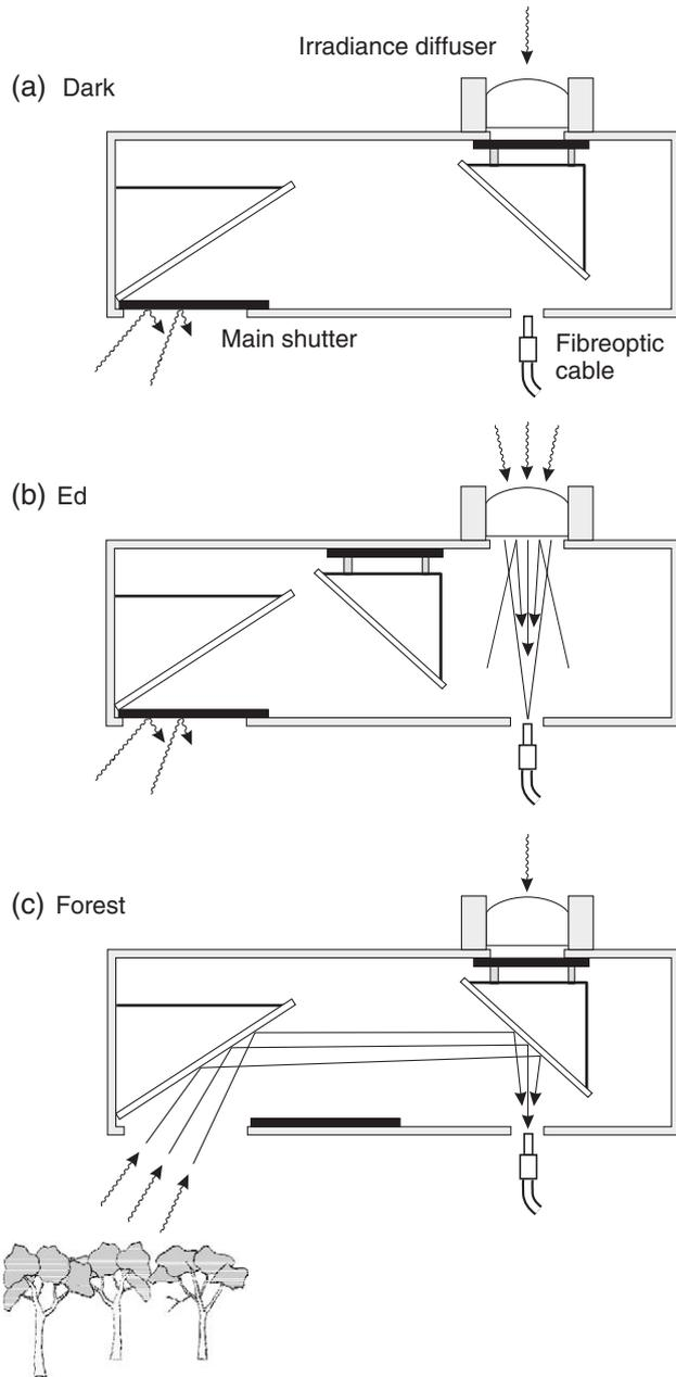
Fig. 2. Mirror and shutter positions for each measurement mode: (a) mirror in home position and shutter closed for measurement of dark current,  $N_0$ ; (b) moveable mirror in position for measurement of incoming irradiance,  $E_d$ ; and (c) moveable mirror in place to measure reflected radiance from forest canopy,  $L_r$ .
